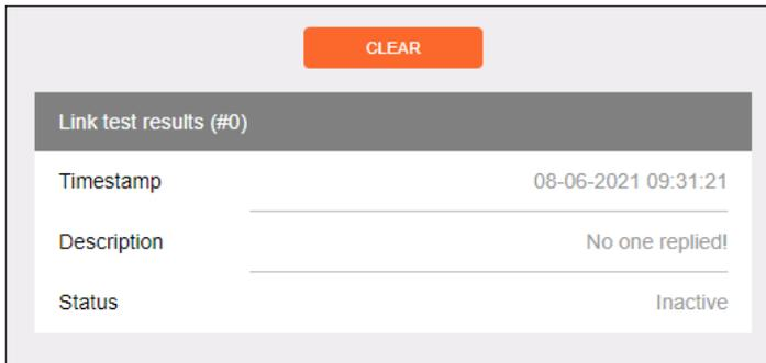
Hovering the mouse over the **Description** field will provide the full IP address of each decoder which received the test, as shown below. If multiple decoders were tested, additional IP addresses will be displayed.
