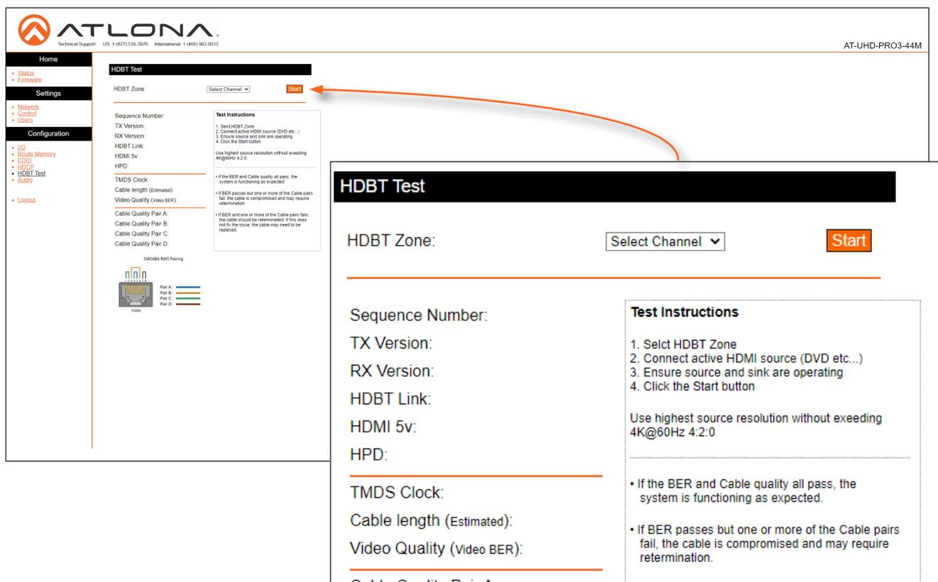
3. Click the **HDBT Zone** drop-down list and select the desired zone to test. Before testing a zone, make sure that an Ethernet cable is connected between the **ZONE OUT** port and a compatible receiver.
