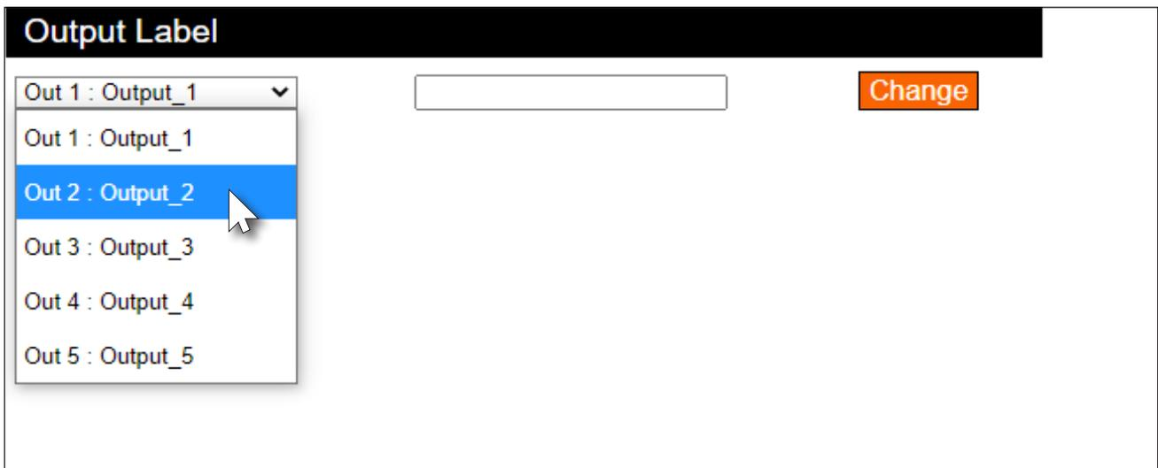
4. Enter the desired name of the input in the **Output Label** field. When entering the name of the output, spaces and special characters are not permitted. In this example, **Out 2 : Output\_2** is being renamed as **4KUHD\_Display**.
