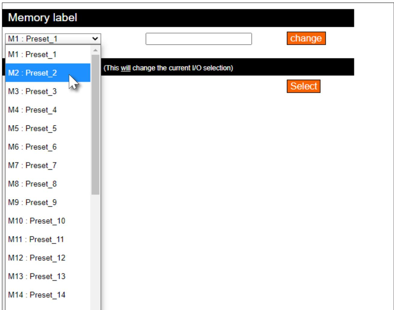
4. Enter the name of the preset in the **Memory label** text field, as shown in the example below.
