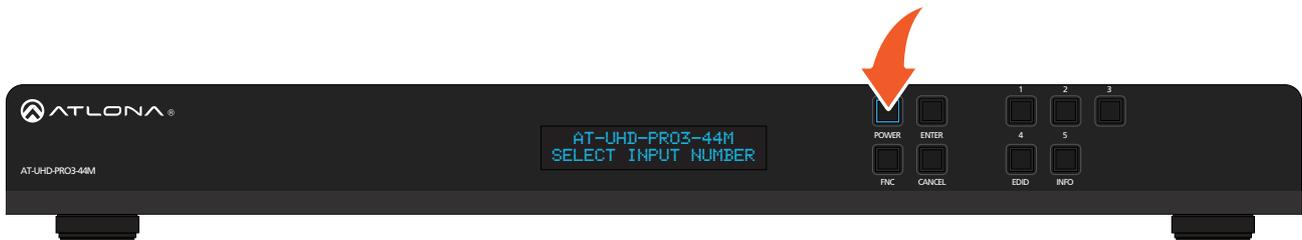
The matrix will power-down and be placed in a low-power state and the **POWER** button will be backlit by a solid red light.
