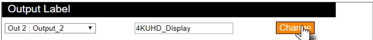
The new name will now be displayed when an output is selected, as shown. Note that if an output is selectable (**Output\_5** drop-down lists), then it will also appear in the drop-down list.
