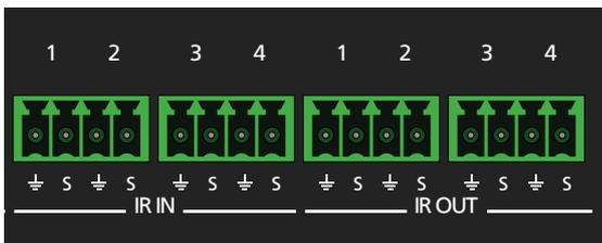
3. Insert the GND and Signal leads into correct terminal, as shown, and tighten the screws to secure each wire. Do no overtighten.
