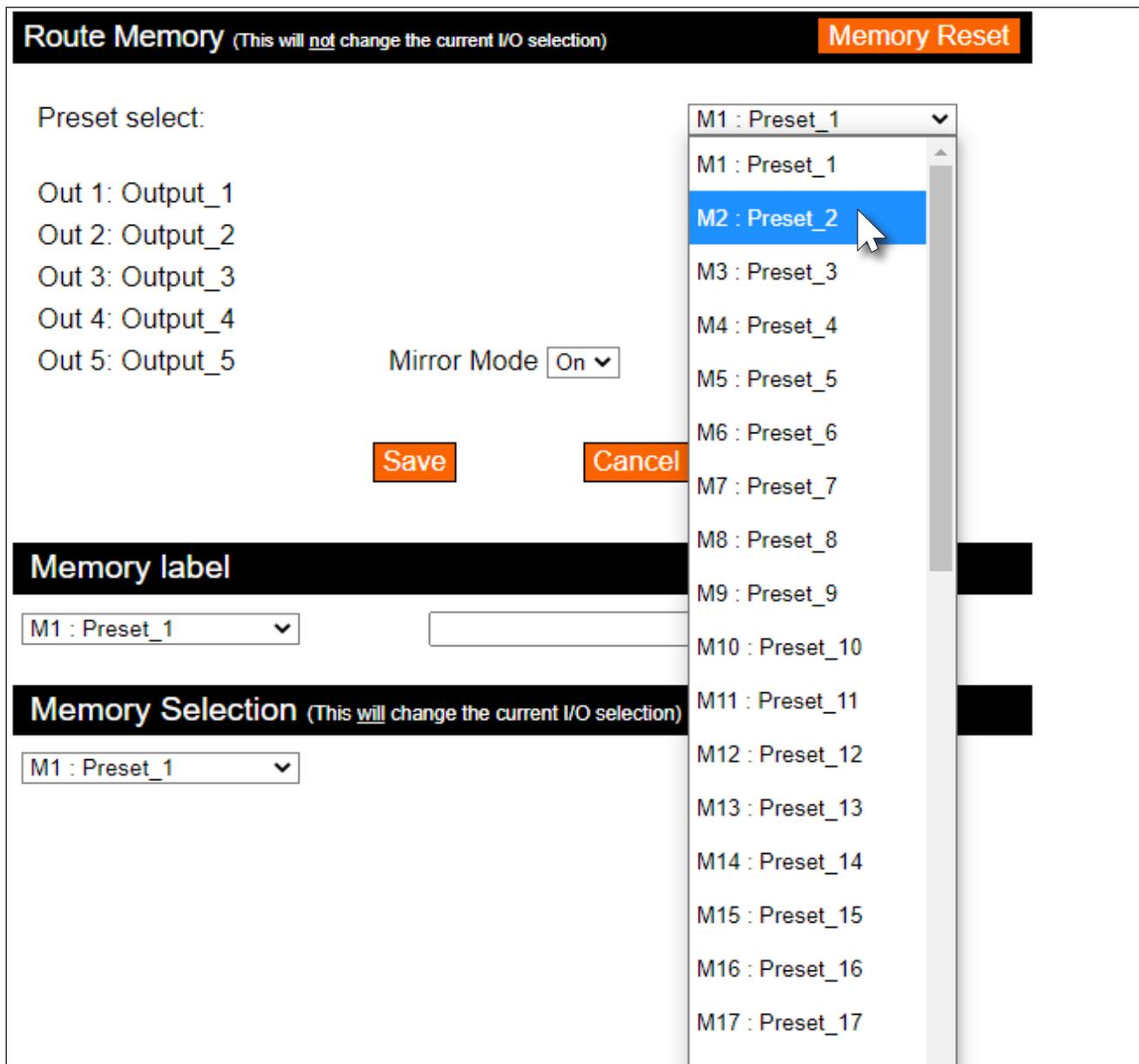
4. Click the drop-down list, next to each output, to set the new routing state. For more information on how to modify routing states, refer to [Routing Inputs to Outputs \(page 21\)](#) and [Audio Routing \(page 31\)](#).
