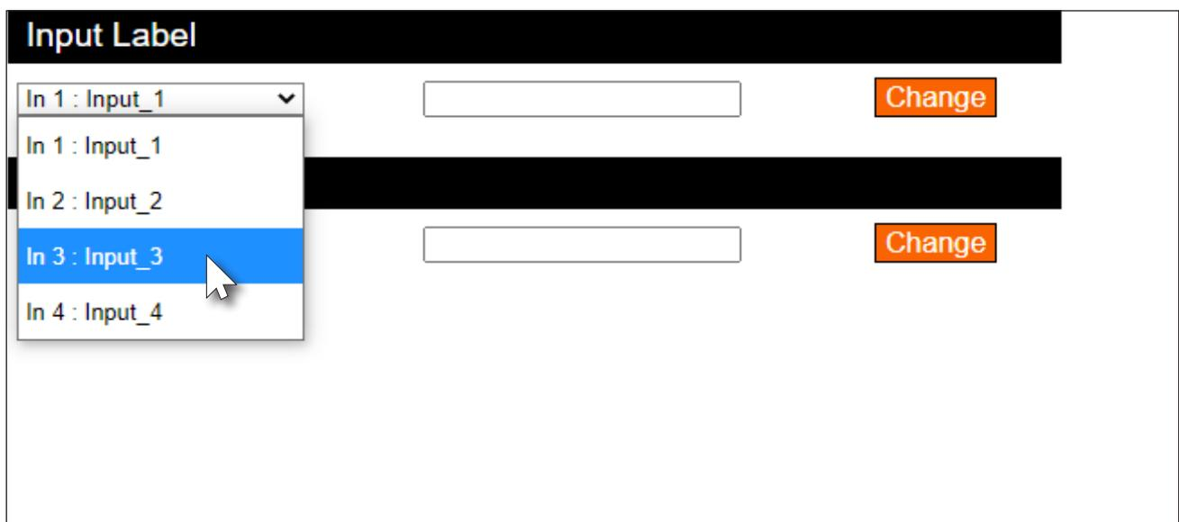
4. Enter the desired name of the input in the **Input Label** field. When entering the name of the input, spaces and special characters are not permitted. In this example, **In 3 : Input\_3** is being renamed as **Blu-ray\_Player**.
