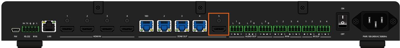
This HDMI port is used to mirror (duplicate) an HDBaseT output signal on the HDMI output port. By default, mirroring is enabled on this port. However, mirroring can be disabled. When mirroring is disabled, any of the four HDMI inputs can be routed to this HDMI output, transforming this product into an 4 x 5 matrix switcher. The default mirror setting is listed below.
