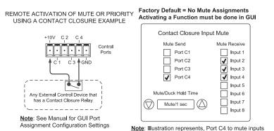
2,3,4, when C4 is activated by connecting C4 to +10V.
