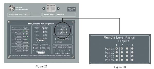
3. Note: Each channel of the DPA can have separate remote levels or all channels combined together onto one level control.
