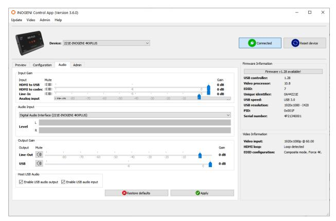
Input Gain: Control of audio gain for HDMI and Line-In.
