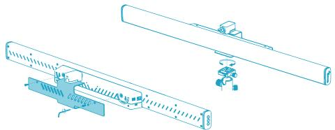
Step 1 (Optional) Fasten a video camera to the Tripod Mount.
