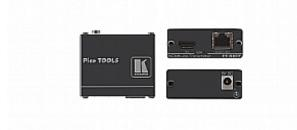
The PT-580T is a 4K resolution, HDBaseT twisted pair transmitter for HDMI signals. The unit inputs an HDMI signal that it converts to a twisted pair signal. An HDBaseT receiver (for example the TP-580R or WP-580R) converts the twisted pair signal back into an HDMI signal and together they form a transmitter receiver pair.
