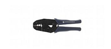
Kramer's precision Crimping Tool is used for terminating bulk coax cable with Kramer's crimp connectors. The multi-format die attaches the three most common connector/cable sets used in professional AV including RG-6, RG-59, and 26/28AWG high-resolution mini coax (RG-179).
