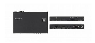
The Kramer VP-427A is a receiver/scaler for HDBaseT twisted pair, HDMI, bidirectional RS-232 and IR signals. The unit receives an HDBaseT signal that it converts to HDMI, IR and RS-232 signals. It up- or down-scales the picture to match the resolution of the HDMI monitor. It includes a simultaneous analog audio output of the embedded HDMI audio.
