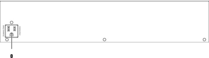
O. Accessory outlet – AC outlet for powering accessories. This outlet is not surge protected or metered.
