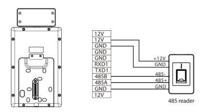
**Note:** 485A and 485B can be connected to the barrier gate or the 485 reader, but cannot be connected to the gate and the reader at the same time.
