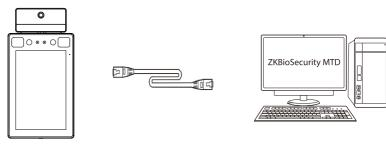
Default IP address: 192.168.1.201 Subnet mask: 255.255.255.0 IP address: 192.168.1.130 Subnet mask: 255.255.255.0
